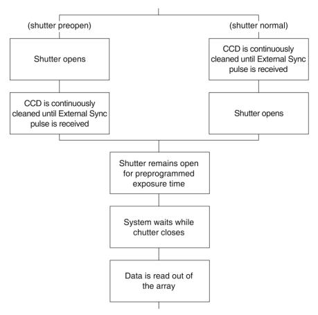
Figure 32. Continuous Cleans {Clean Until Trigger} Flowchart
